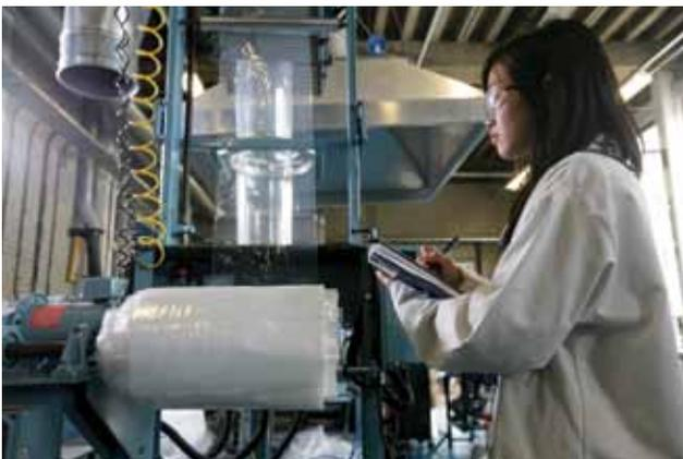
Seow Chin is a PhD student and is shown working on a blown film extrusion machine.
